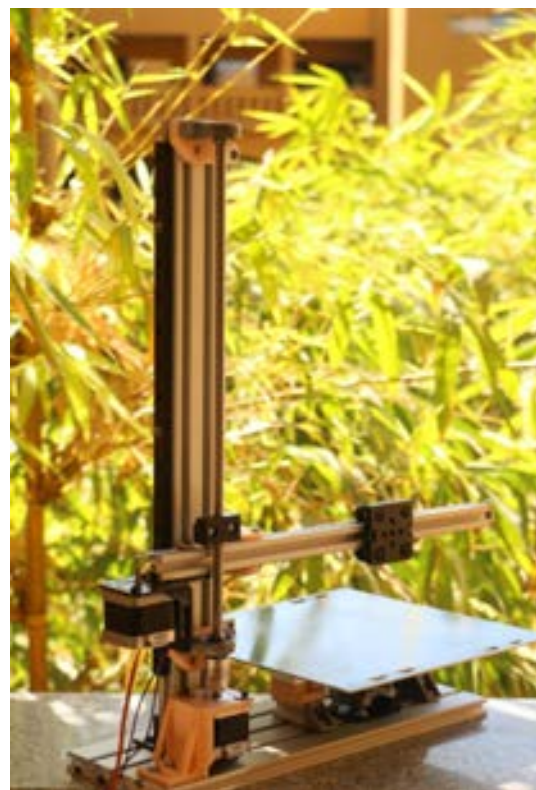
3D printer developed by students of Mechatronics Department, MUJ
